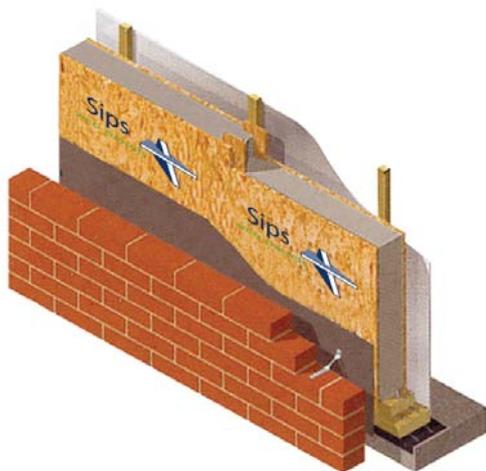
**3. Acoustics** – this bulletin covers the improved sound performance levels that can be delivered by SIP panels. SIPS contribute to improved airborne sound insulation for floors roofs, external, internal and separating/ party/ compartment walls. Much like timber studwork, SIP panels rely on the mass and continuity of plasterboard linings to provide the majority of the sound
