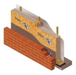
**3. Acoustics** – this bulletin covers the improved sound performance levels that can be delivered by SIP panels. SIPS contribute to improved airborne sound insulation for floors roofs, external, internal and separating/ party/ compartment walls. Much like timber studwork, SIP panels rely on the mass and continuity of plasterboard linings to provide the majority of the sound
