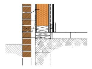
It is important to keep the base of the building above external ground level to mitigate the risk of ground water coming into contact with the SIP. It is recommended that the lowest structural timber (usually the sole plate) is at least 150mm above external ground level and level or above finished floor level. This is also a requirement of some warranty providers.
